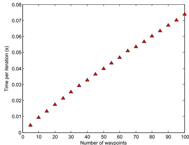
Fig. 12. Average runtime per iteration for different numbers of waypoints in a path.
