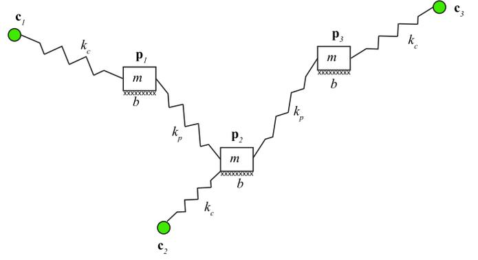
Fig. 8. Illustration of how the path is modeled as a mass-spring-damper system.
