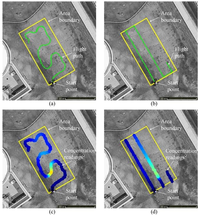
Fig. 18. Flight paths from small area experiments. (a) Flight path flown by the chemical-sensing robot platform during real-world testing based on the path generated using the VPG method. (b) Flight path based on the generated lawnmower path. (c) Concentrations of the Gaussian plume along the flight path generated using the VPG method. (d) Concentrations along the lawnmower flight path.
