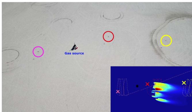
Fig. 1. Three quadcopter aerial robots with chemical sensors scanning an area to generate chemical concentration maps [11]. In this case, the source is a simulated propane leak. CPP methods are important in such applications to optimize the mapping process when robot flight time (energy) is limited.
