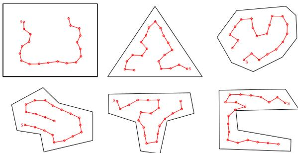
Fig. 11. Examples of paths generated by the VPG algorithm in both convex and nonconvex polygons, using 20 waypoints. Start points are denoted with an “S.”
