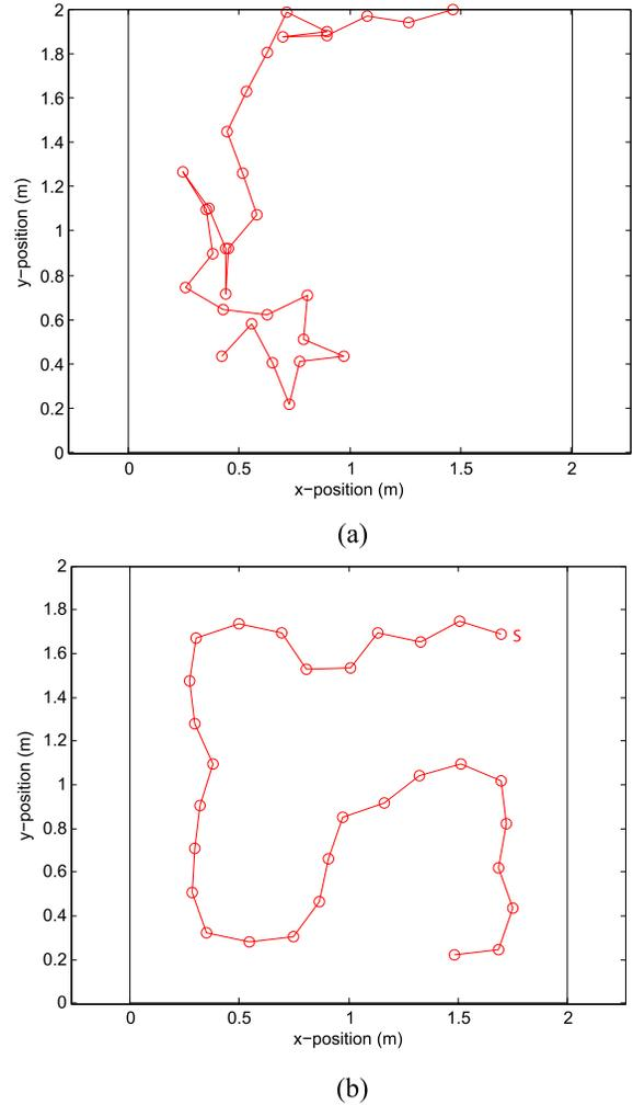
Fig. 10. Path generated using a 2 m  $\times$  2 m area and 30 waypoints with the spacing of 0.2 m. (a) Initial waypoint locations. (b) Final path with the starting point marked with an “S.”
