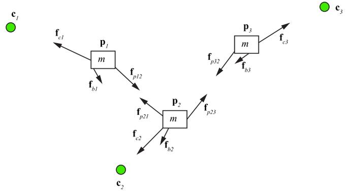
Fig. 9. Free body diagram for a path modeled as a mass-spring-damper system.
