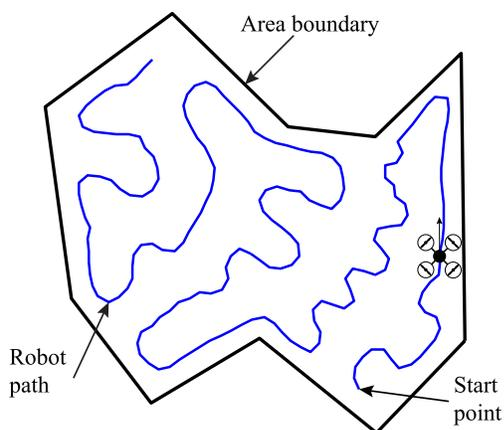
Fig. 2. Example of a near-optimal partial coverage path created by the VPG algorithm given a path-length constraint based on an energy model of a mobile robot.
