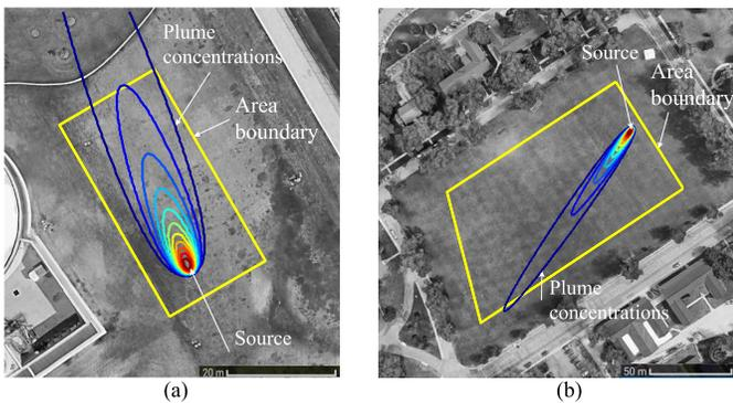
Fig. 17. Gaussian plume model in (a) small and (b) large areas.
