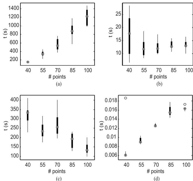
Fig. 14. Average total times to converge for (a) *fmincon*, (b) VPG method, (c) Soltero method, and (d) lawnmower path generation method for different numbers of path waypoints.
