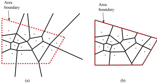
Fig. 6. Illustration of (a) unbounded Voronoi diagram and (b) bounded Voronoi diagram, where the red dashed line represents the area the Voronoi diagram is being bounded to.
