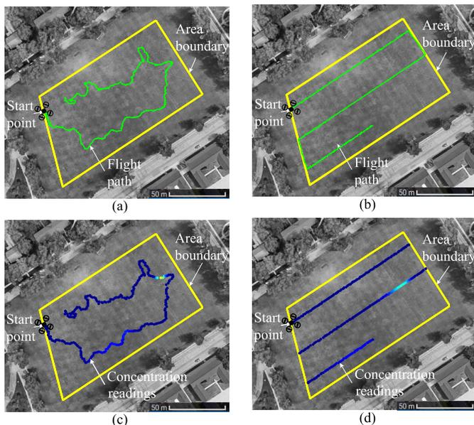
Fig. 19. Flight paths from large area experiments. (a) Flight path flow by the chemical-sensing robot platform during real-world testing based on the path generated using the VPG method. (b) Flight path based on the generated lawnmower path. (c) Concentrations of the Gaussian plume along the flight path generated using the VPG method. (d) Concentrations along the lawnmower flight path.
