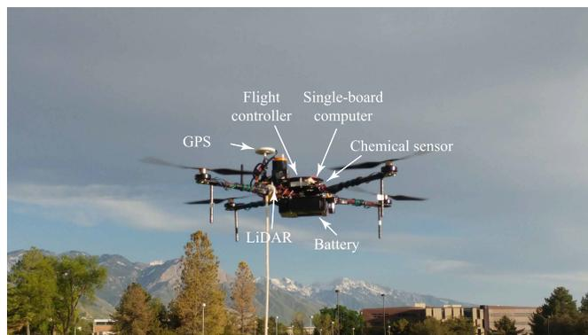
Fig. 15. Enif autonomous chemical-sensing UAV [11] photographed during an in-flight path generation test. Image also shows key components of the system.
