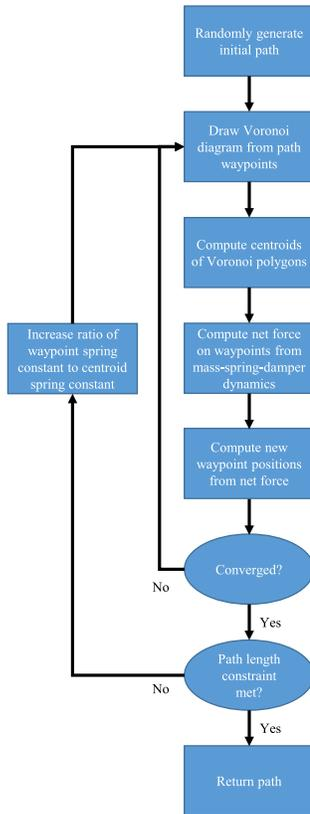
Fig. 5. Flowchart illustrating the high-level VPG algorithm process.
