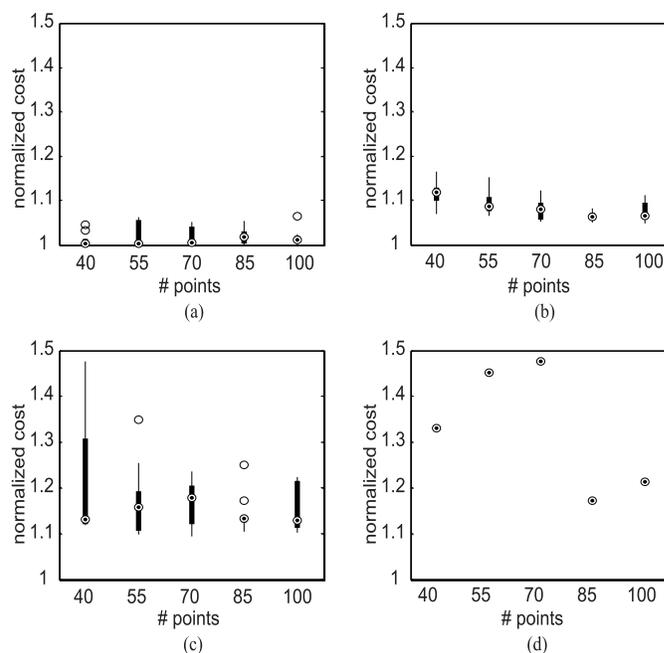
Fig. 13. Costs of the final paths generated by (a) *fmincon*, (b) VPG method, (c) Soltero method, and (d) lawnmower path generation method, normalized by the cost of the actual optimal path for each number of path waypoints, which is assumed to be the lowest cost path found by direct optimization.
