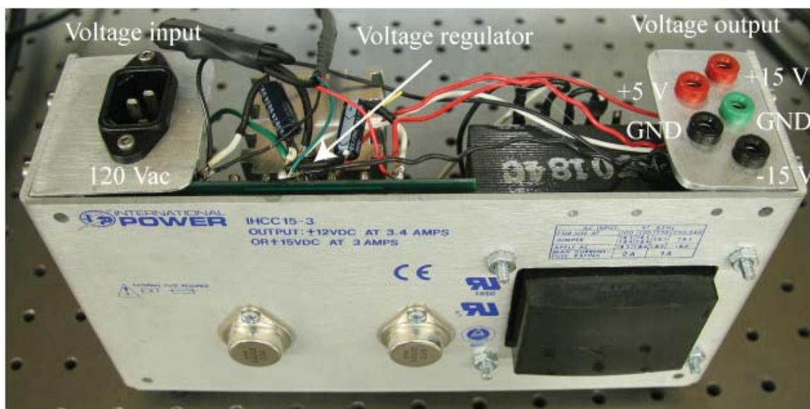
Figure 3.10: Power supply for AFM circuits and voltage references
