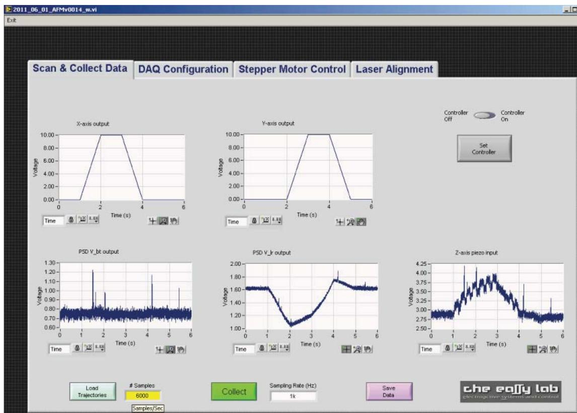
Figure 3.15: LabVIEW AFM program: AFM imaging screen.
