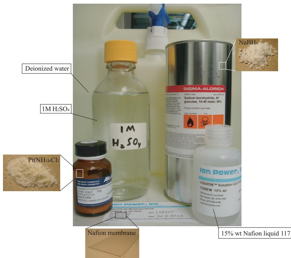
Figure 5.1: The chemicals used to fabricate IPMC actuators, where the Nafion liquid (Ion Power, type 117) was used to cast Nafion membranes, and the other chemicals, including deionized water, 1 molar  $H_2SO_4$ ,  $Pt(NH_3)_4Cl_2$  powders, and  $NaBH_4$  granules, were used for plating electrodes on the surfaces of the Nafion membranes.
